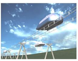
Fig. 4. High-speed module, travel speed – up to 400 km/hour, carrying capacity – 30...60 passengers
