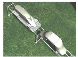
Fig. 5 Freight echelon for bulk freights, speed – up to 150 km/hour, mass – up to 1,000 t
