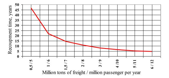
Fig. 9. Dependence of recoupment period of capital investments in route construction "Abu Dhabi — Dubai — Sharjah" (138 km) on the size of freight and passenger flows
