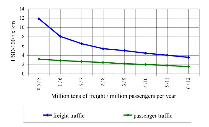
Fig. 10. Dependence of the net cost of traffic along the route "Abu Dhabi — Dubai — Sharjah" (138 km) on the size of freight and passenger flows
