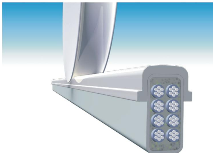
Fig. 9. Wheel on a string-rail
