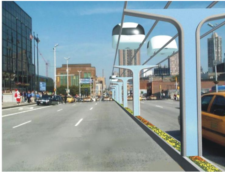
Fig. 1. Double-track UST route in the centre of a city street (speed up to 100 km/hour)
