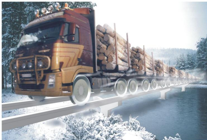
Fig. 3. Freight UST train on the base of a serial truck (mass up to 500 t, speed up to 100 km/hour)
