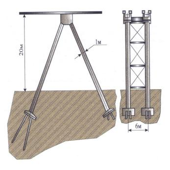
Fig. 19. Anchor support of a double-track STU route
