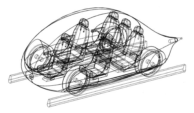
Fig. 39. Design alternative of a high-speed 6-seat passenger vehicle
