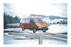
Fig. 6. Mini-bus on string-rails
