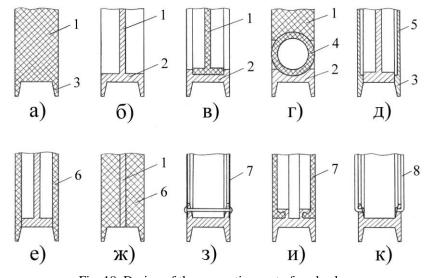
Fig. 18. Design of the supporting part of a wheel: a), b) — solid (monolithic) wheel; c), d), h), i), j) — combined with a moving rim; e), f), g) — combined with moving flanges; 1 — wheel body; 2 — rim; 3 — flange; 4 — elastic toroidal component; 5 — flexible plate; 6 — flexible disk; 7 — membrane; 8 — spoke.
