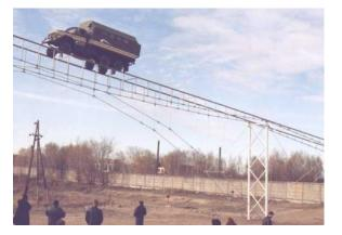
Fig. 42. Modified ZIL-131 on a 48 m string span (November, 2003)
