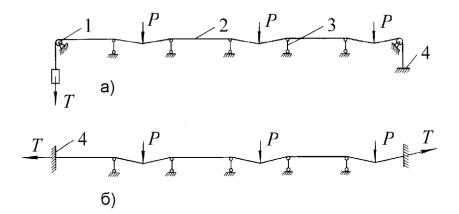
Fig. 17. String linear scheme: a) with a block at the end of a string; b) with a string sealed off; 1 — block; 2 — string; 3 — swing support; 4 — fixing (anchor).
