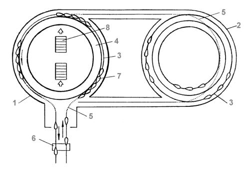
Fig. 26. Scheme of a ring terminal: 1 — terminal building; 2 — depot building; 3 — ring track; 4 — ring-shaped moving platform; 5 — switch; 6 — terminal anchor support; 7 — vehicle; 8 — entrance (exit) to the terminal.
