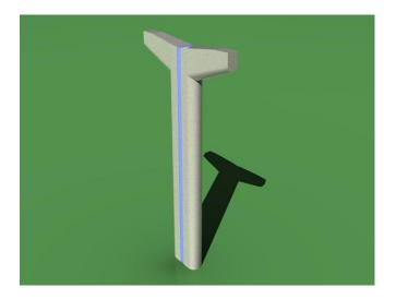
Fig. 20. Small-height intermediate support of a single track STU route
