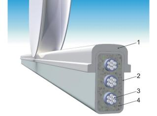
Fig. 13. Two-rim steel wheel on a string-rail: 1 — rail head; 2 — body; 3 — string; 4 — concrete
