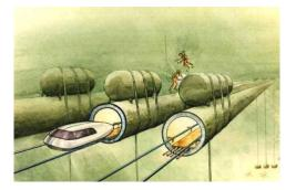
Fig. 34. Design alternative of a marine section of STU route
