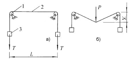
Fig. 16. String block system: a) without external load; b) with a load; 1 — block; 2 — string; 3 — load.
