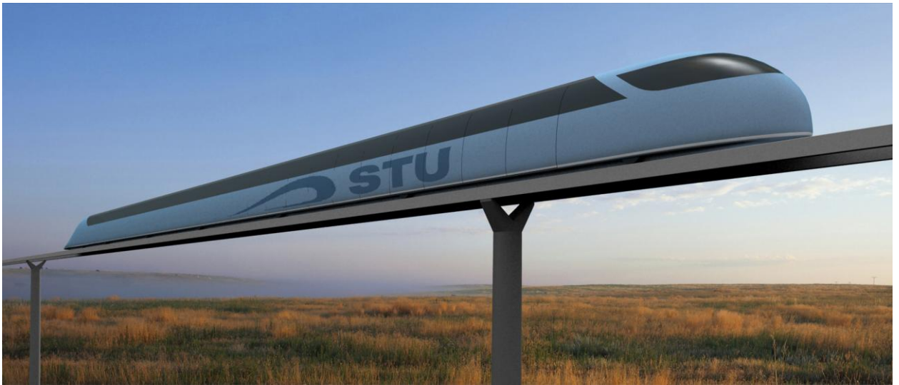
Fig. 2. High-speed way STU Speed up to 360 km/h, gauge 0,75 m
