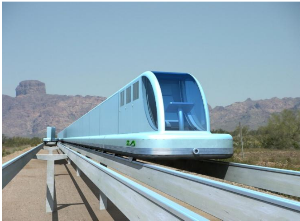
Fig. 1. Supported STS 50 MTPA (STM with load capacity of 160 tons).
