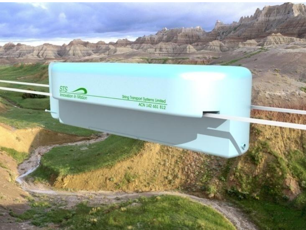
Fig. 2. Suspended STS 30 MTPA (STM with load capacity of 8 tons)
