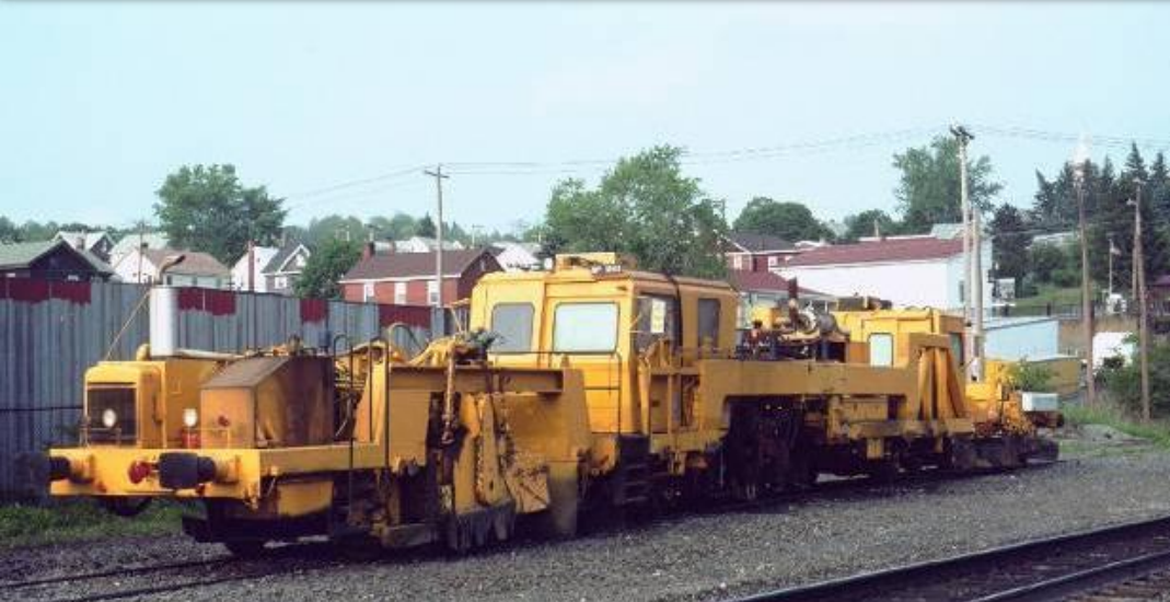
Examples of ballast and embankment requirements for conventional rail and a ballast tamper. A ballast tamper is used to repack ballast under a rail track and its sleepers and is an example of the type of equipment and industry that has been developed purely to support the high maintenance requirement for conventional rail systems.
