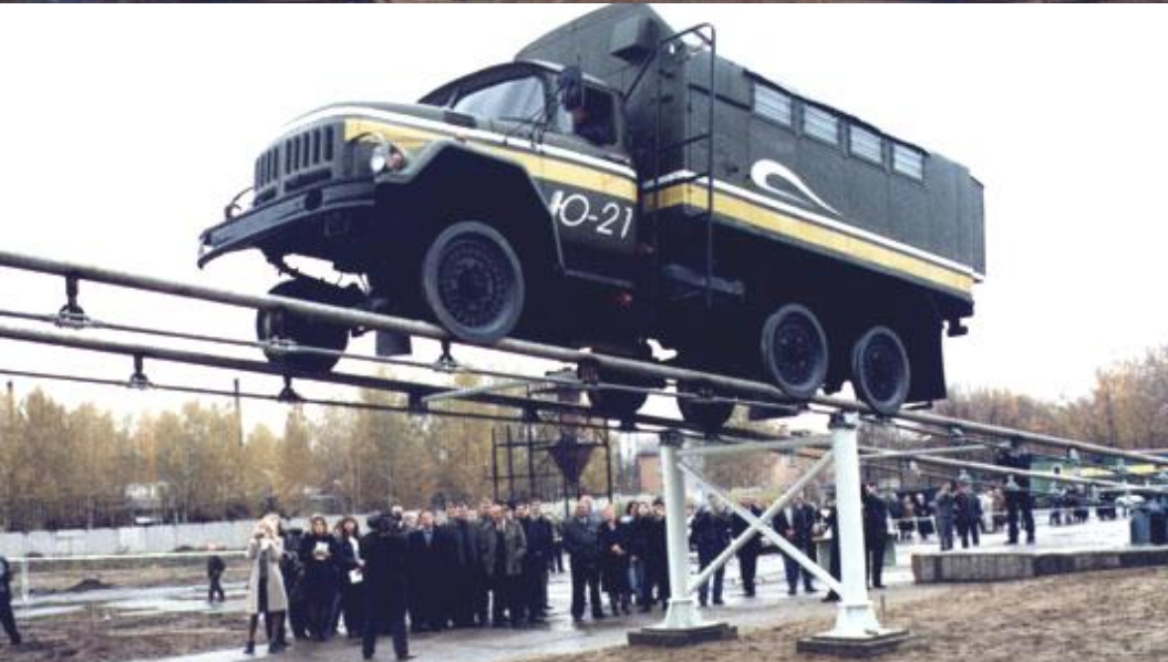
Testing of full scale segment of string rail track
