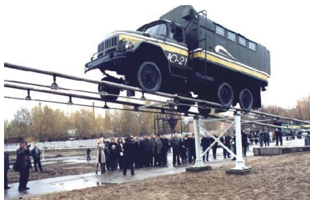
String Transport full scale test track
