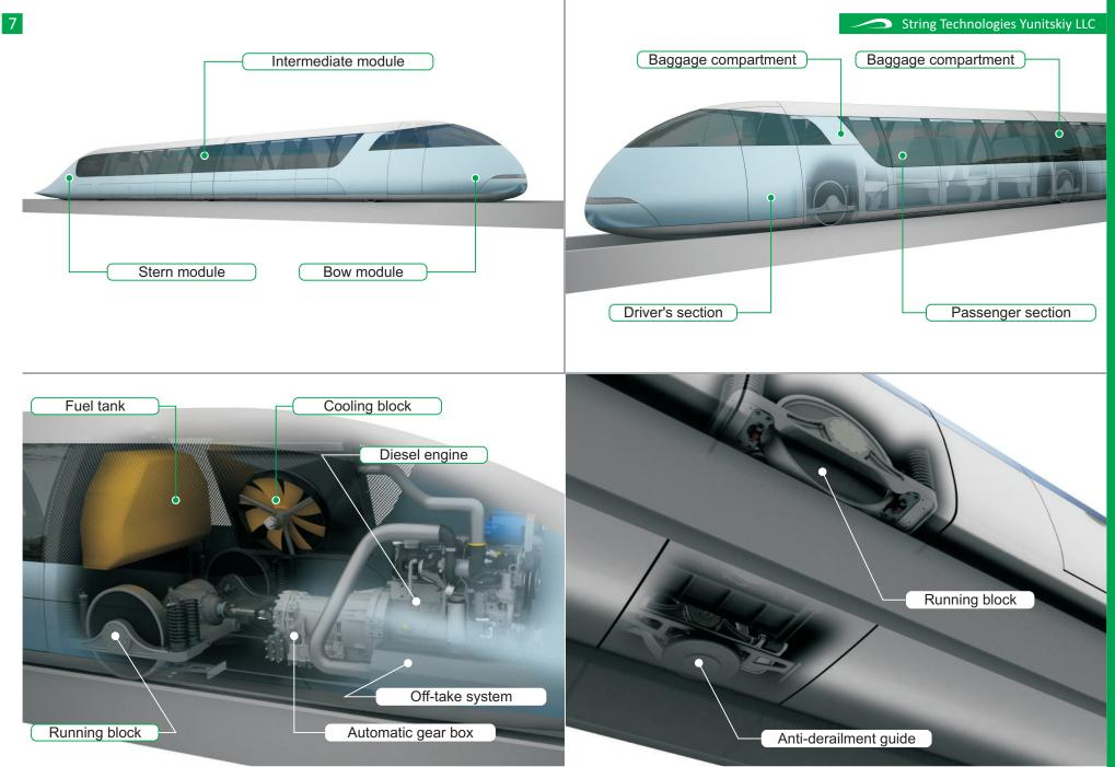
High-speed passenger diesel-electric STY train
