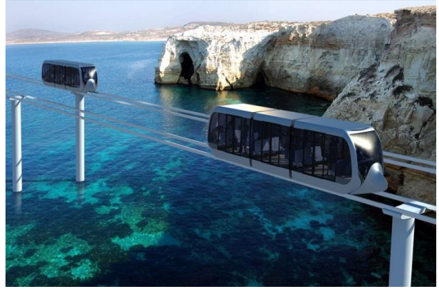
Fig. 4. Passenger SkyWay railcars— unibuses (left – high-speed intercity running at up to 500 km/h, right – city transit, up to 150 km/h)
