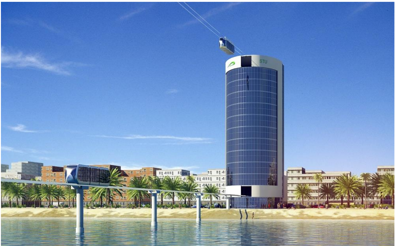
Fig. 31. Linear City fragment featuring two SkyWay transport systems — horizontal lifts — mounted (elevation about 10 m) and suspended (elevation about 100 m)
